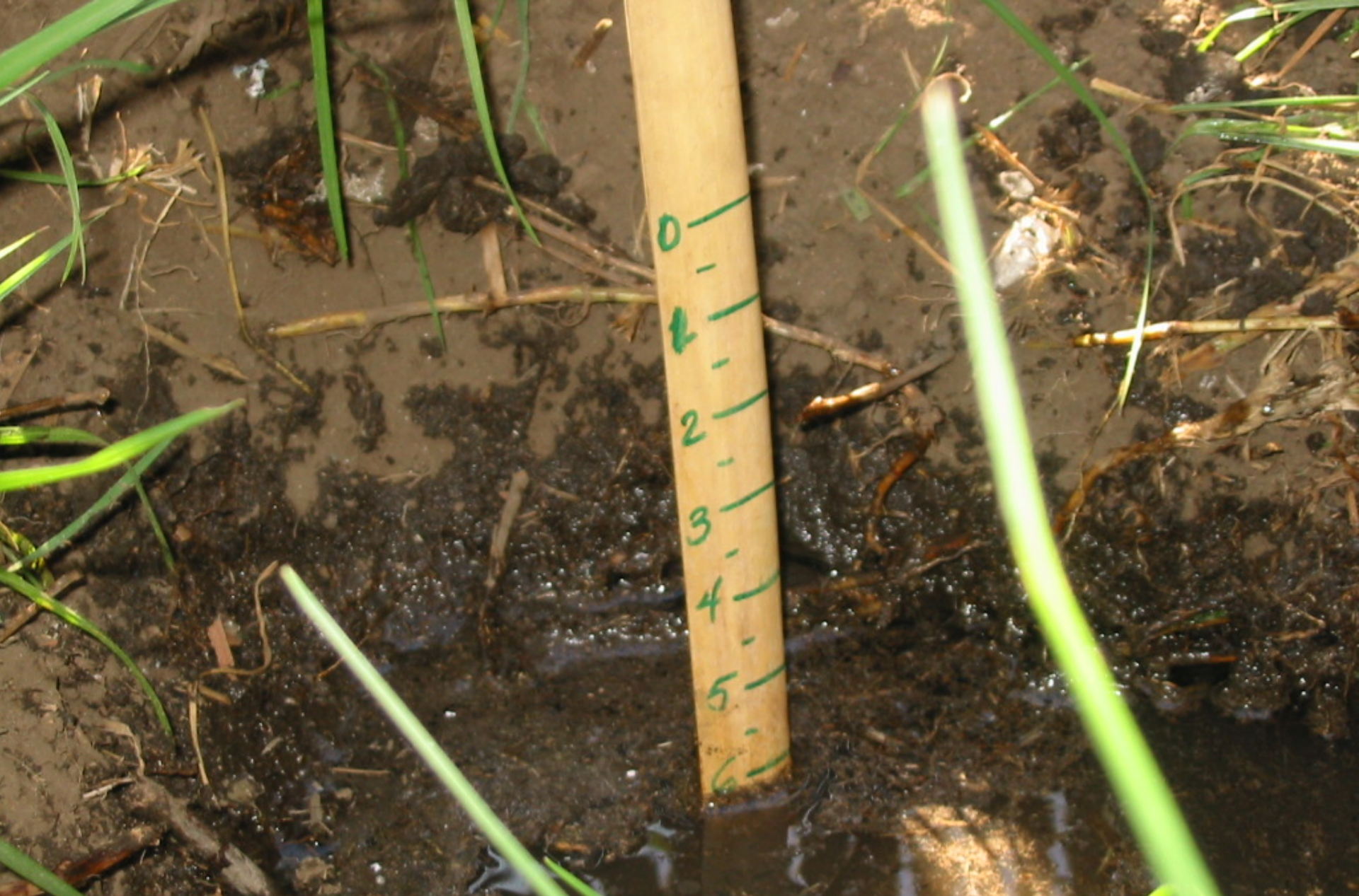
Measure how fast it drains. This Oakland soil drained 2 ½" per hour. Clay soil might drain at only ¼" per hour.
