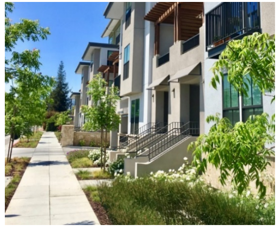
Fig. A.6: Access to ground floor residential units from the sidewalk using stoops.
