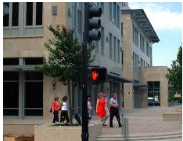
Fig. H.22: Both small and large-scale new development should preserve the rhythm and fine-grained pedestrian scale of existing buildings within the Historic Retail District by respecting the relatively narrow building increments, which are predominantly 25' to 50'.
