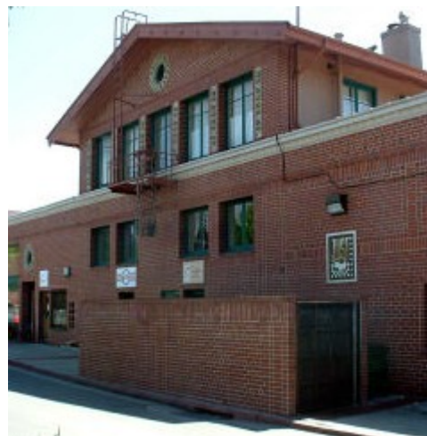
Fig. H.20: Service facilities should be screened with enclosures and devices consistent with the building architecture.
